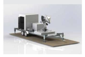
The E750 is also available in turn key truck and trailer mounted mobile configurations.
